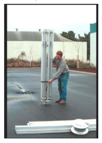
3. Gently squeeze the vertical support members and the roof trusses together to release the chained locking pins. Lower the vertical members to the ground. Extend the telescoping roof trusses until the outermost locking buttons snap into place.
